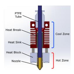
*Note*. This is an image showing what the hot end assembly looks like in the Ender 5 S1. From Creality Experts, n.d, https://www.crealityexperts.com/bimetallic-heatbreak-install-hot-end
